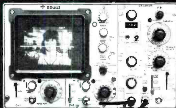
Or it can display the complete picture, with a bright line indicating the line under examination.
